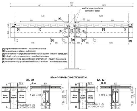
Fig. 2. Scheme of the tested elements
