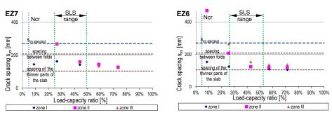
Fig. 8. The average crack spacing - specimens with the extended end-plate connections
