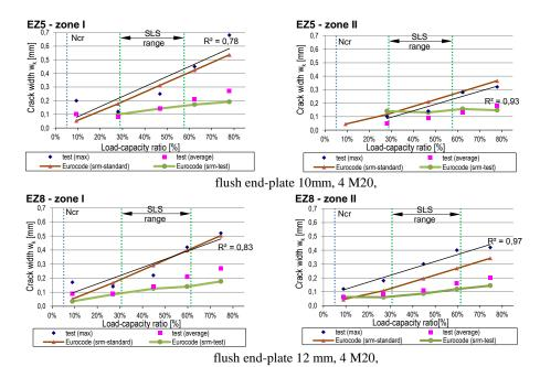
Fig. 9. The crack spacing - specimens with the flush end-plate connections
