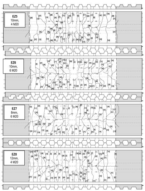
Fig. 5. The view of cracks on the surface of the slab directly before failture
