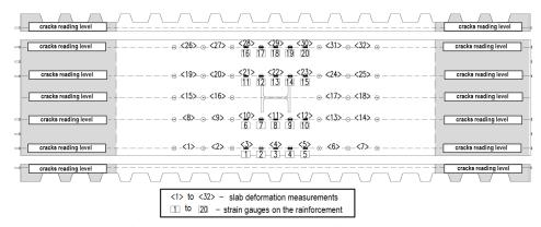
Fig. 3. The view of the tested slab - the distribution of benchmarks on the slab surface, the strain gauges on the reinforcement and crack width reading levels
